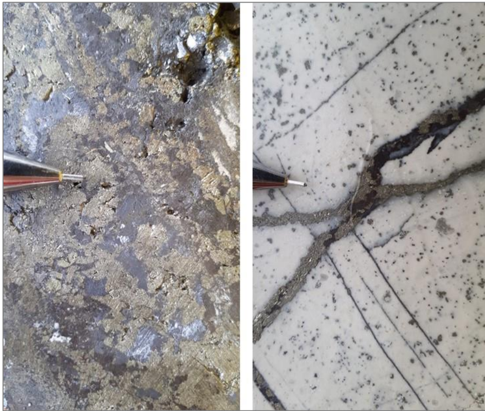
Figure 3: Left image: Segment of massive sulphide vein from CC19-06, 351 m depth composed of chalcopyrite, sphalerite, marcasite, tetrahedrite. Right image: Example of mineralized rhyolitic dike host rock from CC19-06.
